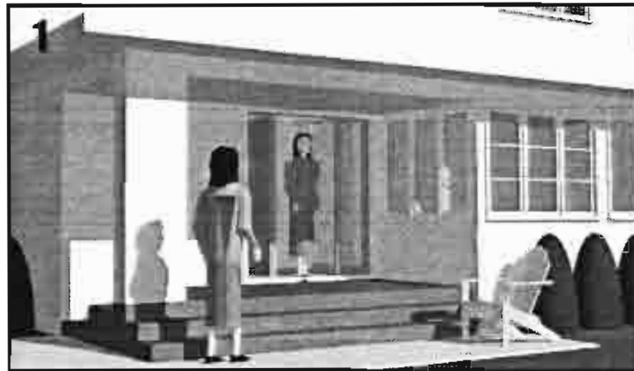
1 SOCIAL STAIRS RULE: There must be a place to socialize at the front door of the house, ideally wide and shallow stairs where people can hang out.
