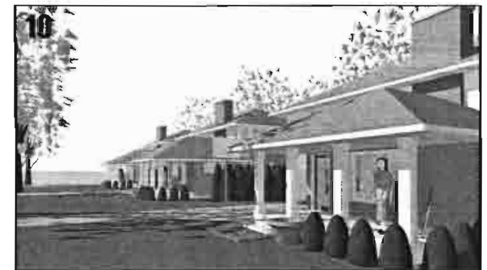
8 PARALLEL FACE RULE: The long side or face of the house must run parallel to the street to help define the free-flowing front yards so characteristic of Fridley.
