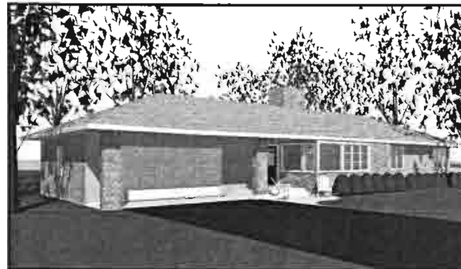
HORIZONTAL RULE: The house must be long and low and horizontal and close to the ground. Ideally the main level should be no more than 12"-18" above grade.
