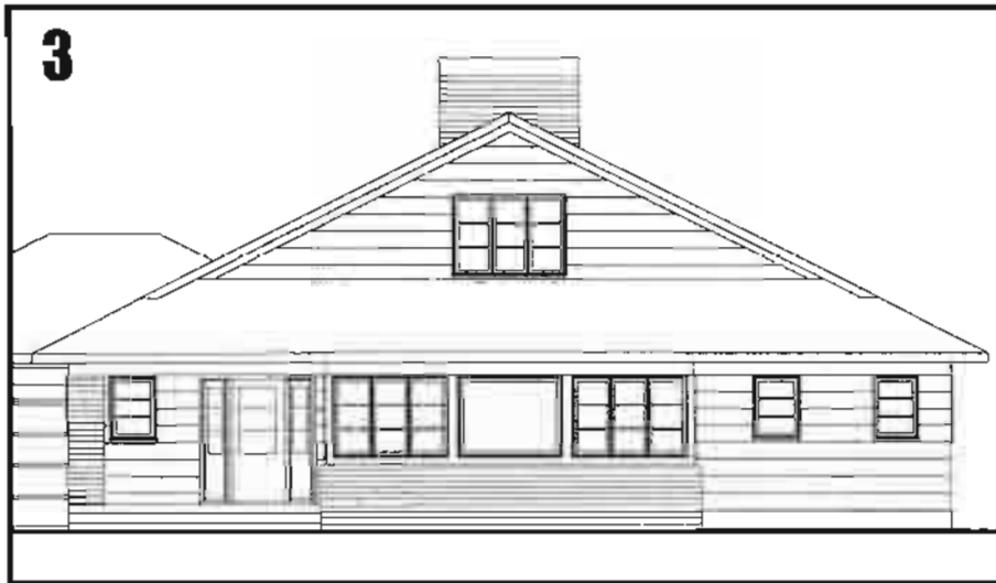
3 WINDOW PROPORTIONS RULE: Window proportions must be largely horizontal. The sashes on double-hung windows must have horizontal proportions, and casements (except in bathrooms and closets) must be mulled together in groups with horizontal proportions.
