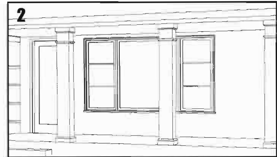
2 FEATURE WINDOW RULE: There must be a feature window, such as a large picture window with flankers or a corner window, which is the focus of the front elevation.
