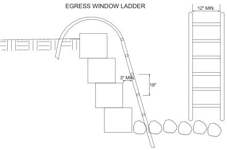
LADDERS OR RUNGS SHALL HAVE AN INSIDE WIDTH OF AT LEAST 12 INCHES, SHALL PROJECT AT LEAST 3 INCHES FROM THE WALL AND SHALL BE SPACED NOT MORE THAN 18 INCHES ON CENTER VERTICALLY FOR THE FULL HEIGHT OF THE WINDOW WELL.
