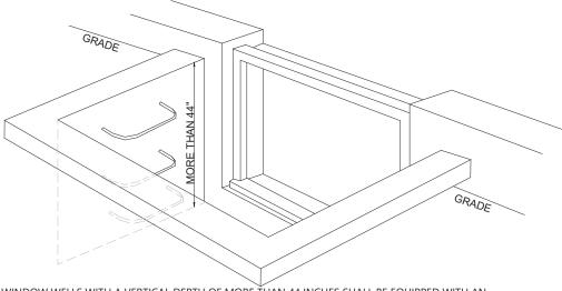
WINDOW WELLS WITH A VERTICAL DEPTH OF MORE THAN 44 INCHES SHALL BE EQUIPPED WITH AN APPROVED PERMANENTLY AFFIXED LADDER OR STAIRS THAT ARE ACCESSIBLE WITH THE WINDOW IN THE FULLY OPEN POSITION. THE LADDER OR STAIRS SHALL NOT ENCROACH INTO THE REQUIRE DIMENSIONS OF THE WINDOW WELL BY MORE THAN 6 INCHES.
