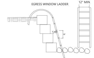
LADDERS OR RUNGS SHALL HAVE AN INSIDE WIDTH OF AT LEAST 12 INCHES, SHALL PROJECT AT LEAST 3 INCHES FROM THE WALL AND SHALL BE SPACED NOT MORE THAN 18 INCHES ON CENTER VERTICALLY FOR THE FULL HEIGHT OF THE WINDOW WELL.
