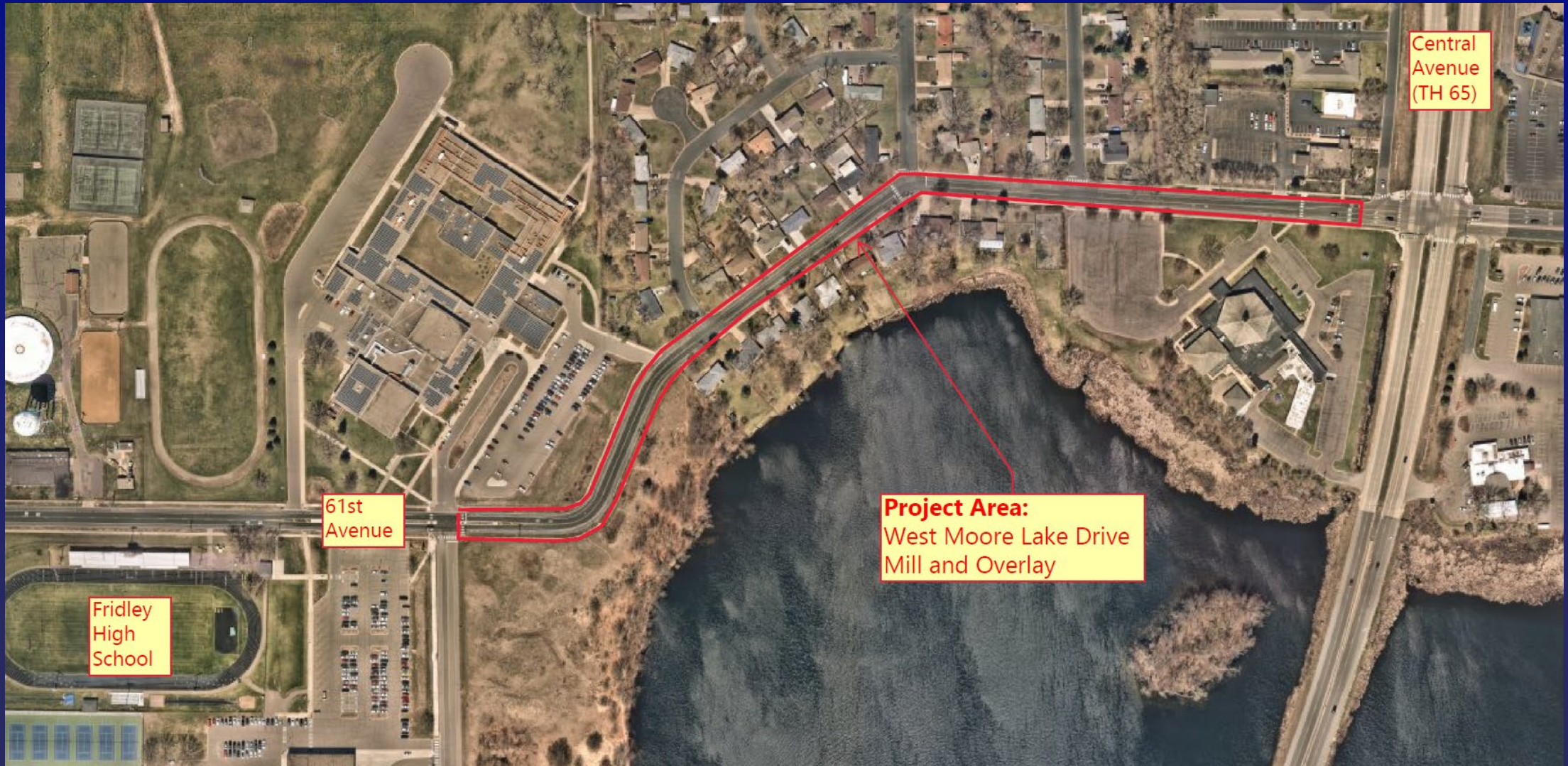
West Moore Lake Drive Mill and Overlay
